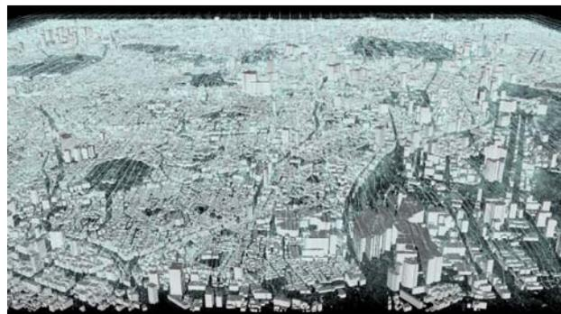
Figure 2. Snapshot of wind flow using particles with a  $10,080 \times 10,240 \times 512$  mesh on a  $10 \text{ km} \times 10 \text{ km}$  urban area of Tokyo.
