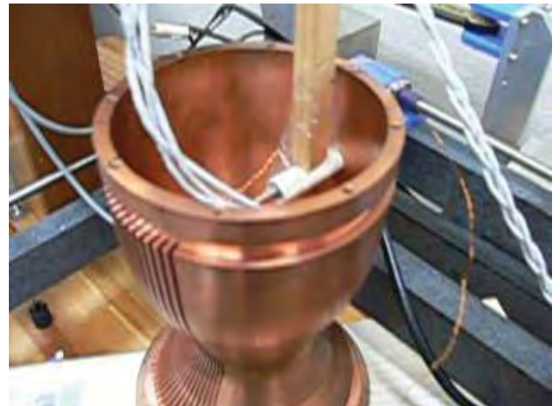
Copper alloy chamber with grooves and defects
